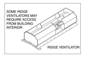
Vents that do not have moving parts will require very little maintenance. Ventilators containing moving parts such as pulleys, rollers or cranks for flue operation will require periodic lubrication at pivot points. Simple operation from time to time will aid in breaking corrosion loose.
