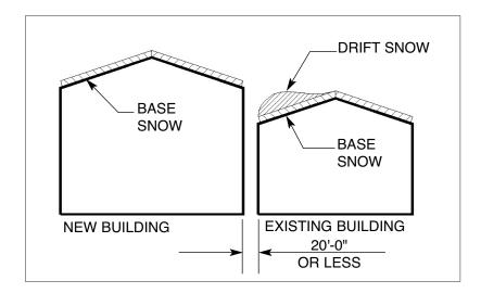
Placing a new taller building adjacent to an existing building can result in snow drift loads on the existing building that were not considered in the original design. The new snow drift load could cause the original building to collapse. When adding a new building within 20 feet of an existing building, the existing building should be checked for potential additional loads and reinforced if necessary.
