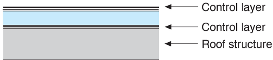
Figure 4: Control Layers in Roof Assemblies – Control layers are provided above and below the thermal control layer. The intent is to keep rain, air and vapor from entering the assembly from the top side and to keep air and vapor from entering the assembly from the bottom side.
