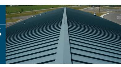
BattenLok® HS is a mechanically field seamed, high strength structural standing seam roof system. The panels have a 2" tall vertical seam and are available in both 12-inch and 16-inch widths. BattenLok® HS can be installed directly over purlins or bar joists, is capable of transitioning from roof to fascia and does not require a solid substructure for support.
